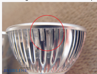
Mounting screw screwed in a separated inner frame
